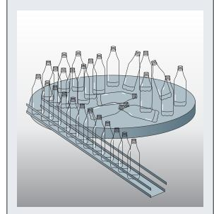
Toppled bottles are uprighted by an orienter based on sensor output as they leave the accumulating table.
