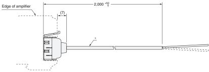
\* E3X-CN12: 2.6 dia. cable / 1 conductor / Standard length: 2 m (Conductor cross section: 0.2 mm² (AWG24), Insulator diameter: 1.1 mm) E3X-CN22: 4 dia. cable / 2 conductors / Standard length: 2 m (Conductor cross section: 0.2 mm² (AWG24), Insulator diameter: 1.1 mm)
