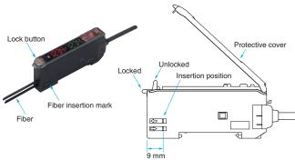
Note: If one of the fibers from the Fiber Unit has a white line, such as with a Coaxial Sensor, that fiber is for the Emitter. Insert it into the Emitter section. Refer to Dimensions for the Fiber Unit to see if there is an Emitter fiber.
