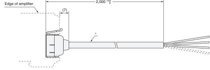
\* E3X-CN11: 4 dla. cable / 3 conductors / Standard length: 2 m (Conductor cross section: 0.2 mm² (AWG24), Insulator diameter: 1.1 mm) E3X-CN21: 4 dla. cable / 4 conductors / Standard length: 2 m (Conductor cross section: 0.2 mm² (AWG24), Insulator diameter: 1.1 mm)
