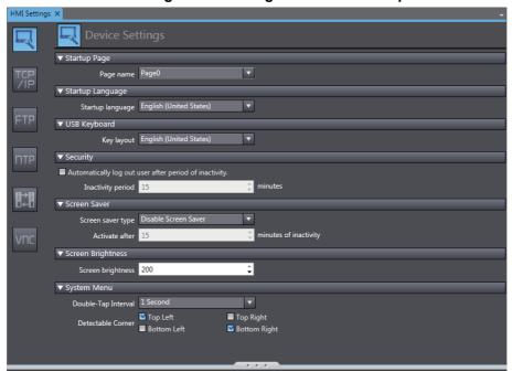
2 Click the TCP/IP Settings Button and set the IP address and other settings for Ethernet port 1 on the TCP/IP Settings Display. Also set the subnet mask and default gateway as required.
