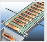
Aperture angle of 15° ensures stable detection even with narrowly spaced workpieces.
