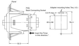
Note: The mounting panel thickness must be 1 to 3.2 mm. \* Insert the Timer from the back of the Adapter.
