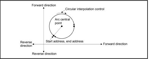
Fig.6.18 Positioning control of a complete round
