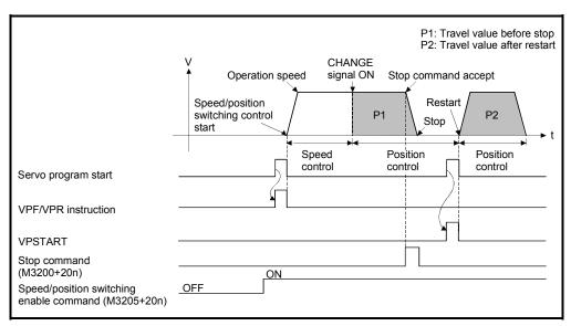
Fig.6.28 Re-starting during speed control
