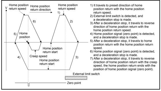
(b) When the zero point is not in the home position return direction.
