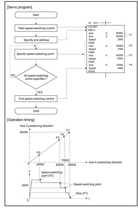
Procedure of the servo program and operation timing
