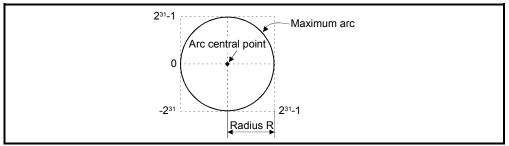
Fig.6.22 Maximum arc radius
