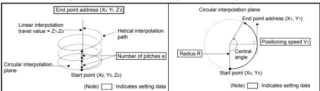
Operation details for absolute radius-specified helical interpolation are shown below.
