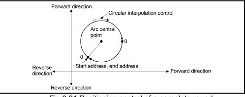
Fig.6.21 Positioning control of a complete round
