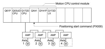
(2) Positioning operation detailsPositioning using the servo program No.0 is shown below.
