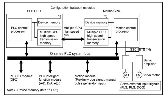
Fig.3.1 Flow of the internal signals/external signals
