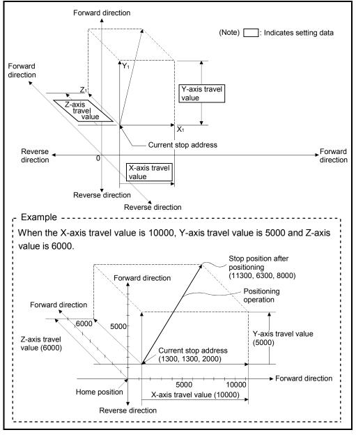
Fig.6.6 Positioning using incremental data method
