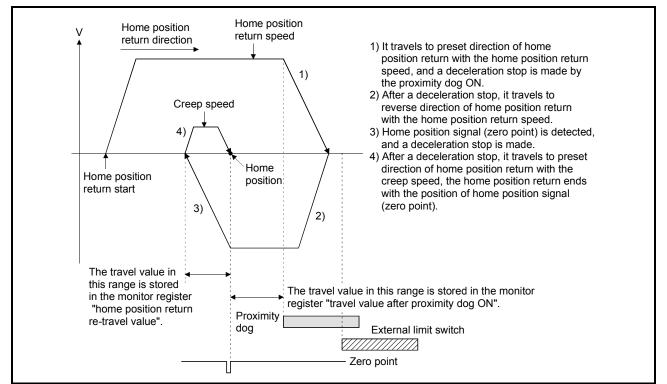
Fig. 6.44 Home position return operation by the scale home position signal detection type
