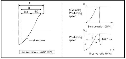
S-curve ratio can be set by the servo program is following two methods.(a) Direct specification
