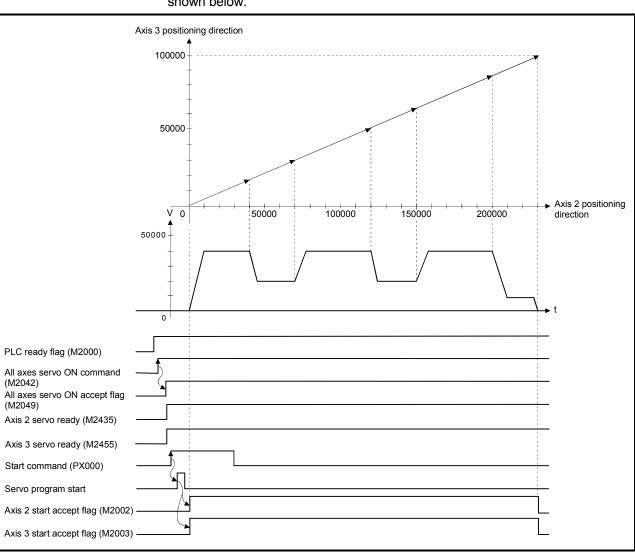
(3) Operation timing and speed-switching positions Operation timing and speed-switching points for speed-switching control are shown below.
