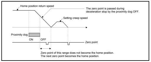
(b) The position executed deceleration stop by the proximity dog OFF is near zero point, a home position discrepancy equivalent to one revolution of the servomotor may occur. Adjust the position of proximity dog OFF, such that the home position return re-travel value becomes half the travel value for one revolution of the servomotor.
