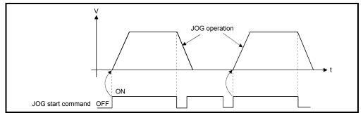
After that, the JOG operation is executed by the JOG start command OFF to ON.
