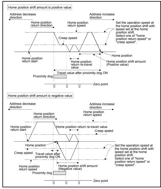
Fig. 6.52 Operation for home position shift
