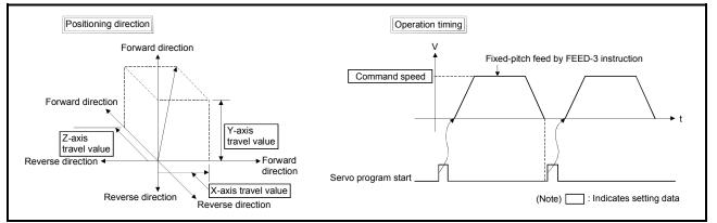
Fig. 6.25 Fixed-pitch feed control using 3 axes linear interpolation
