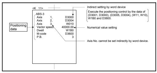
Fig. 5.4 Example of indirect setting by word device for positioning data
