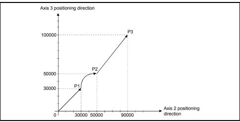
Fig.6.30 Positioning for Axis 2 and Axis 3
