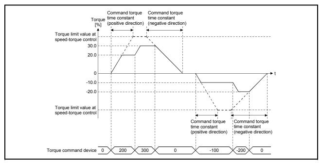
When the torque generation direction of servo motor is changed due to the command torque change during torque control or continuous operation to torque control, the operation is as follows.
