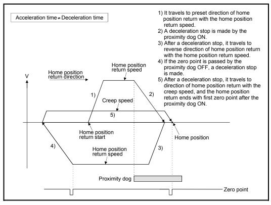
(d) When it starts in the proximity dog, the zero point is not passed at the time of the proximity dog is turned OFF during travel to reverse direction of home position return, it continues to travel with home position return speed until the zero point is passed. The zero point is passed again during deceleration by zero point pass, the home position becomes this side compared with the case to pass zero point at the time of the proximity dog OFF.
