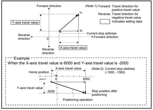
Fig.6.4 Positioning using incremental data method
