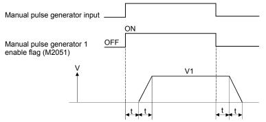
Output speed (V1) = [Number of input pulses/ms] × [Manual pulse generator 1- pulse input magnification setting]
