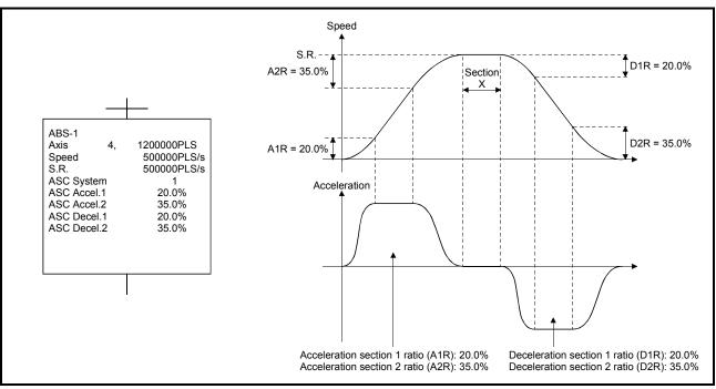
A sample servo program using the advanced S-curve acceleration/deceleration is shown below.
