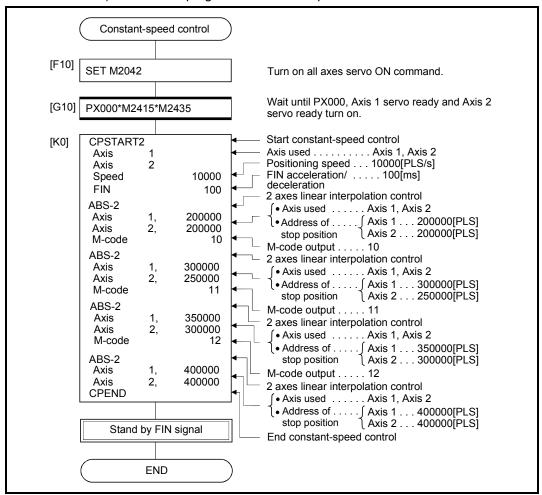
(d) Motion SFC program1) Motion SFC program for constant-speed control is shown below.
