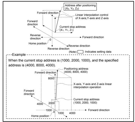
Fig.6.5 Positioning using absolute data method
