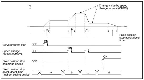
(10) Deceleration speed by the stop command (M3200+20n)/rapid stop command (M3201+20n) is controlled with fixed inclination (deceleration speed).
