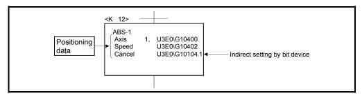
Fig. 5.5 Example of indirect setting by bit device for positioning data
