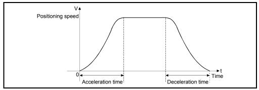
S-curve ratio set the part of the sine curve used to produce the acceleration and deceleration curve as shown in the diagram below.
