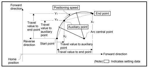
Fig.6.11 Circular interpolation control using incremental data method
