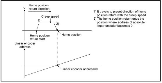
Fig. 6.48 Home position return by the dogless home position signal reference type (Operation C)
