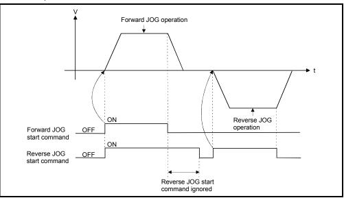
(2) If the JOG start command (M3202+20n/M3203+20n) turns on during deceleration by the JOG start command OFF, after deceleration stop, JOG operation is not executed.
