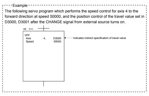
(b) The travel value is stored in the data register for travel value change during speed control in the Motion SFC program. When the CHANGE signal turns on, the contents of the data register for travel value change are set as the travel value.
