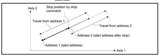
When the address 2 is moved to the same address (address which calculates with start address + specified travel value) using the INCD, the following processing using the servo program and Motion SFC program is required.
