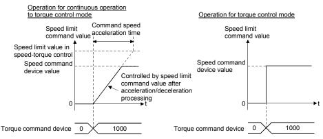
During continuous operation to torque control mode, the torque control is executed at command torque set in "Torque command device". Command torque can be changed any time during continuous operation to torque control mode.
