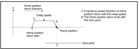
Fig. 6.47 Home position return by the dogless home position signal reference type (Operation B)
