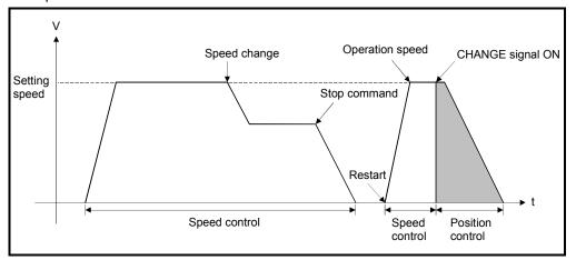
Fig.6.29 Re-starting after speed change
