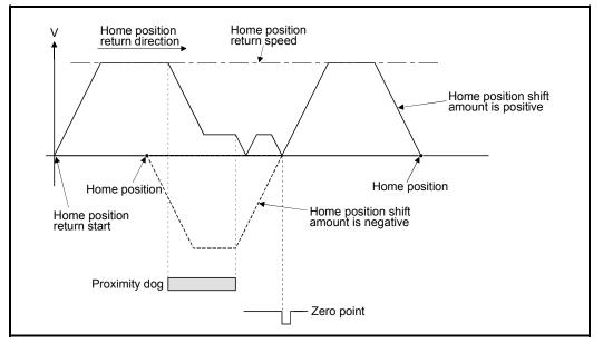
Fig. 6.54 Operation for home position shift with the home position return speed
