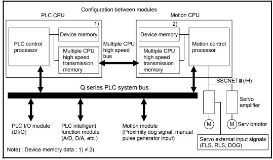
The device memory composition of the Motion CPU and PLC CPU is shown below.
