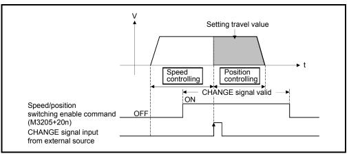
Fig. 6.27 Re-starting during speed control
