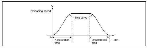
As shown below, the S-curve ratio setting serves to select the part of the sine curve to be used as the acceleration/deceleration curve.
