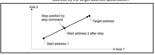
2) For INCD ...... Positioning control of the travel value from the stop address.
