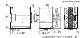
[1] Direct mounting hole:2 holes of 64.5 (0.18") (mounting screw: M4 screw)
