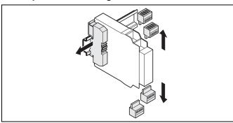
⇒ Remove the removable terminals with wiring and the end clips.
