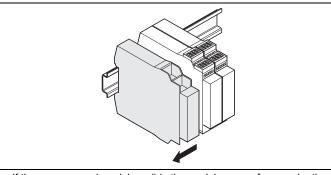
⇒ If there are several modules, slide the modules away from each other individually in the direction of the arrow until the side plug connection is
