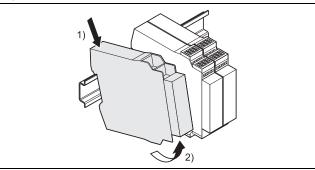
⇒ Press the module downwards at the rear (1)) and remove it from the DIN rail in the direction of the arrow while keeping it pressed down (2)).
