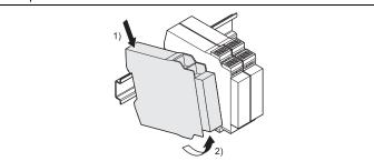
⇒ Press the module downwards at the rear (1)) and remove it from the DIN rail in the direction of the arrow while keeping it pressed down (2)).
