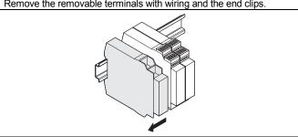
⇒ If there are several modules, slide the modules away from each other individually in the direction of the arrow until the side plug connection is
