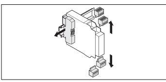
⇒ Remove the removable terminals with wiring and the end clips.
